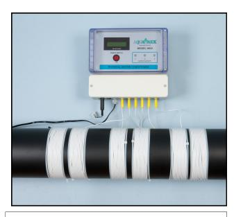
directions from a central point. When facing the pipe, one aerial should start by passing behind the pipe and the other should pass in front of the pipe. Secure each end of the aerial with a cable tie.
