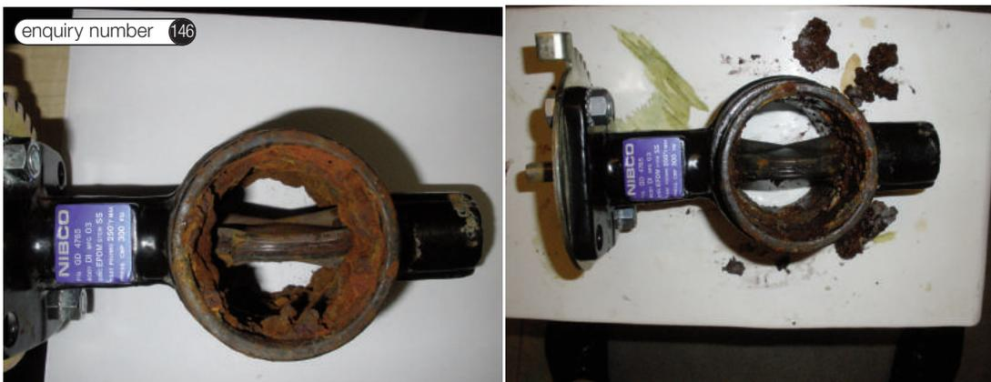
PWCs can remove existing scale encrustation as seen in this valve fitted here. After just 11 weeks the encrusted scale has broken away
