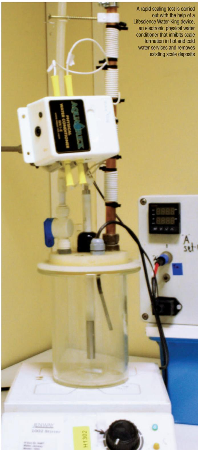
A rapid scaling test is carried out with the help of a Lifescience Water-King device, an electronic physical water conditioner that inhibits scale formation in hot and cold water services and removes existing scale deposits
